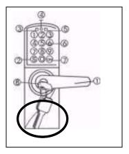
Remove the battery case by inserting the small green screw driver through the bottom hole of the back side of the front mount (see below). As you press the screw driver through the hole the case will release from the bottom of the mount. Place 4 AA batteries in the case and replace the case in the mount.
